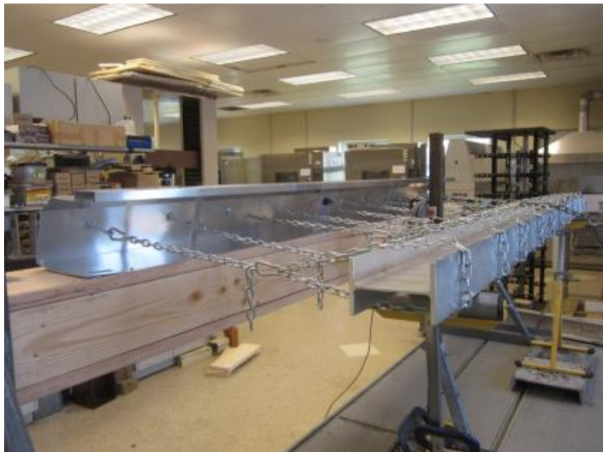
Photo No. 4 ANSI/SPRI Test G-2 Vertical Load
