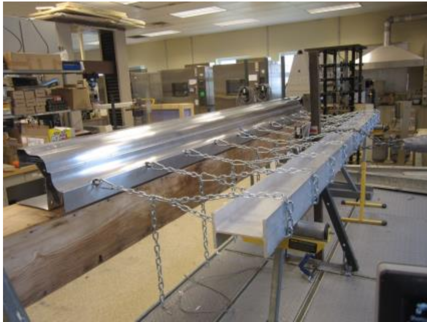
Photo No. 5 ANSI/SPRI Test G-3 Static Load
