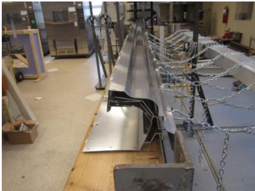
Photo No. 6 ANSI/SPRI Test G-3 Static Load
