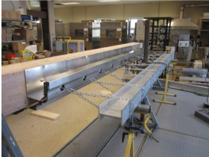
Photo No. 1 ANSI/SPRI Test G-1 Horizontal Load
