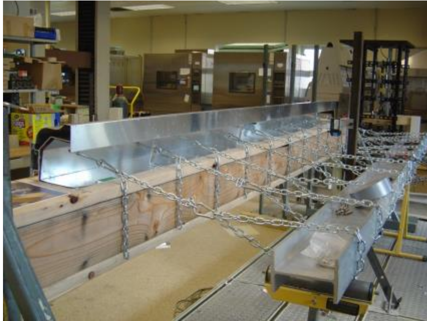
Photo No. 3 ANSI/SPRI Test G-2 Vertical Load
