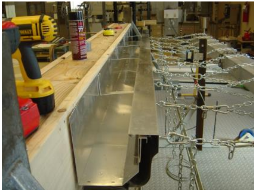
Photo No. 2 ANSI/SPRI Test G-1 Horizontal Load
